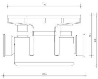
POZZETTO DI TIPO B IN POLIETILENE, CON GRIGLIA IN GHISA SFEROIDALE D400
