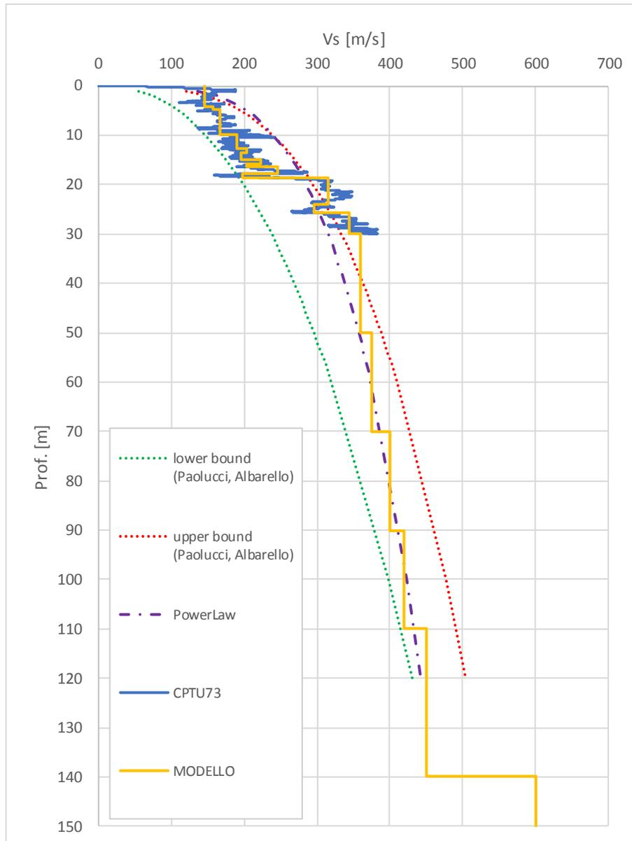
**FIGURA 4-1 - PROFILO DI Vs LUNGO LA VERTICALE DI INDAGINE CPTU 73.**
