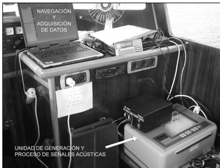
figure 9- Single beam transceiver and navigation/acquisition computer
