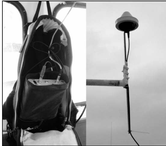
figure 11- Topcon Map-R GD dGPS receiver and csi Wireless CDA-2 dGPS antenna
