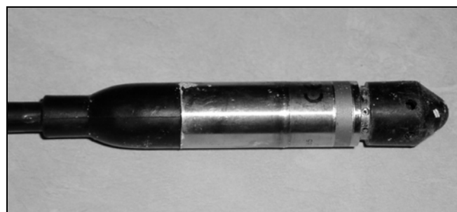
figure 6- Pressure sensor of the Valeport 740 tide gauge
