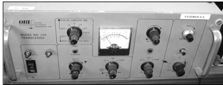
figure 5- Sub-bottom profile transmitter-receiver unit
