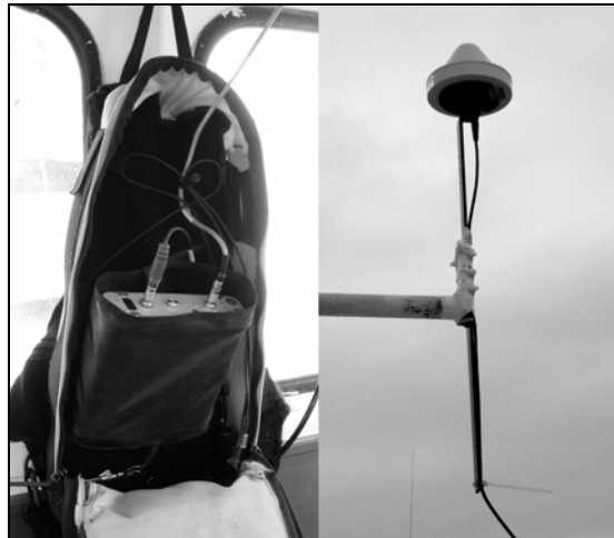
figure 10- Topcon Map-R GD dGPS receiver and csi Wireless CDA-2 dGPS antenna
