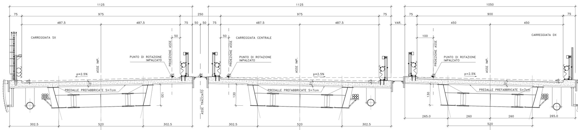
DETTAGLIO TIPOLOGICO APOGGIO PREDALLE IMPALCATO (B=10.50m travi h=130cm)
