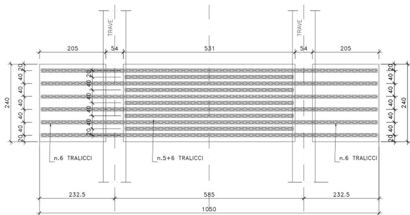
DETTAGLIO TIPOLOGICO APOGGIO PREDALLE IMPALCATO (B=11.25m travi h=130cm)
