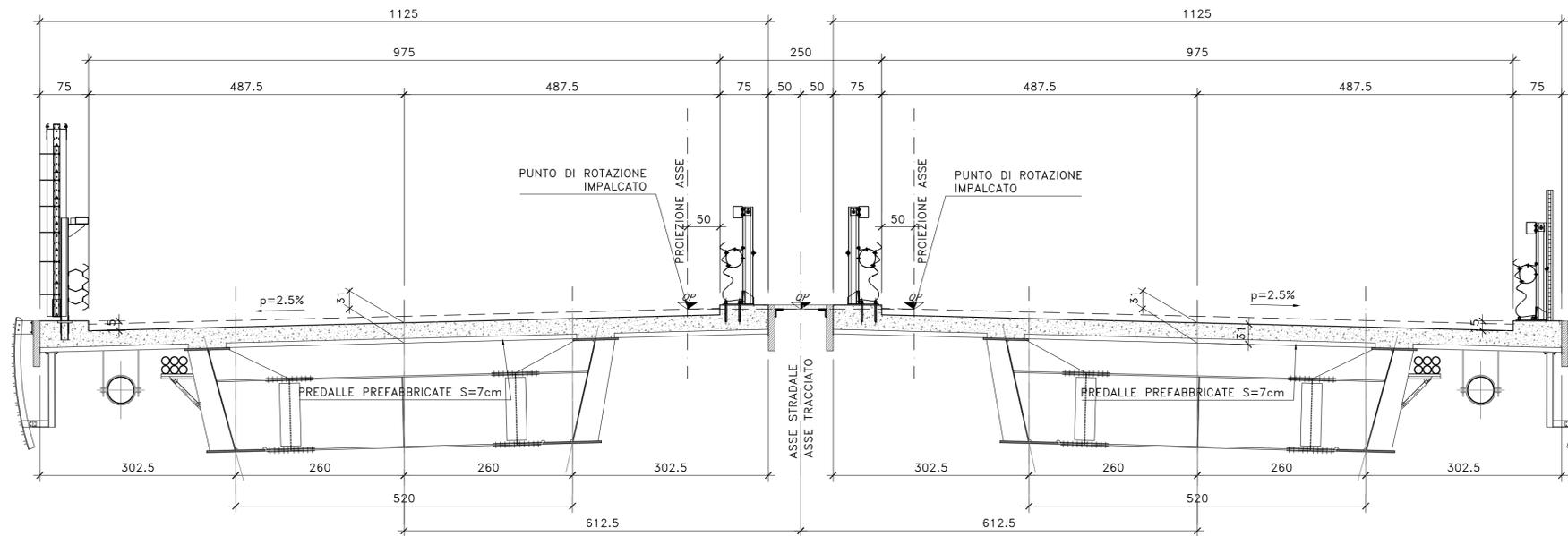
DETTAGLIO TIPOLOGICO APPOGGIO PREDALLE IMPALCATO (B=11.25m travi h160cm)
