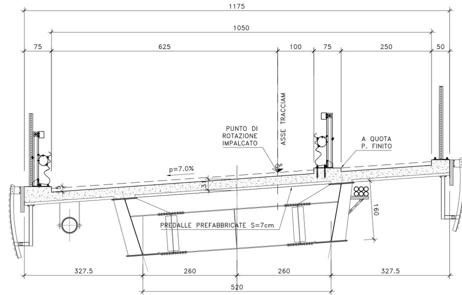
DETTAGLIO TIPOLOGICO APPOGGIO PREDALLE IMPALCATO CV01 (B=11.75m travi h160cm)
