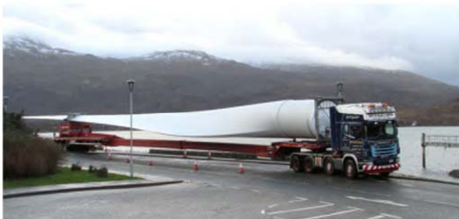
Example of exceptional transport for the blade, in max configuration (about 95 mt).
