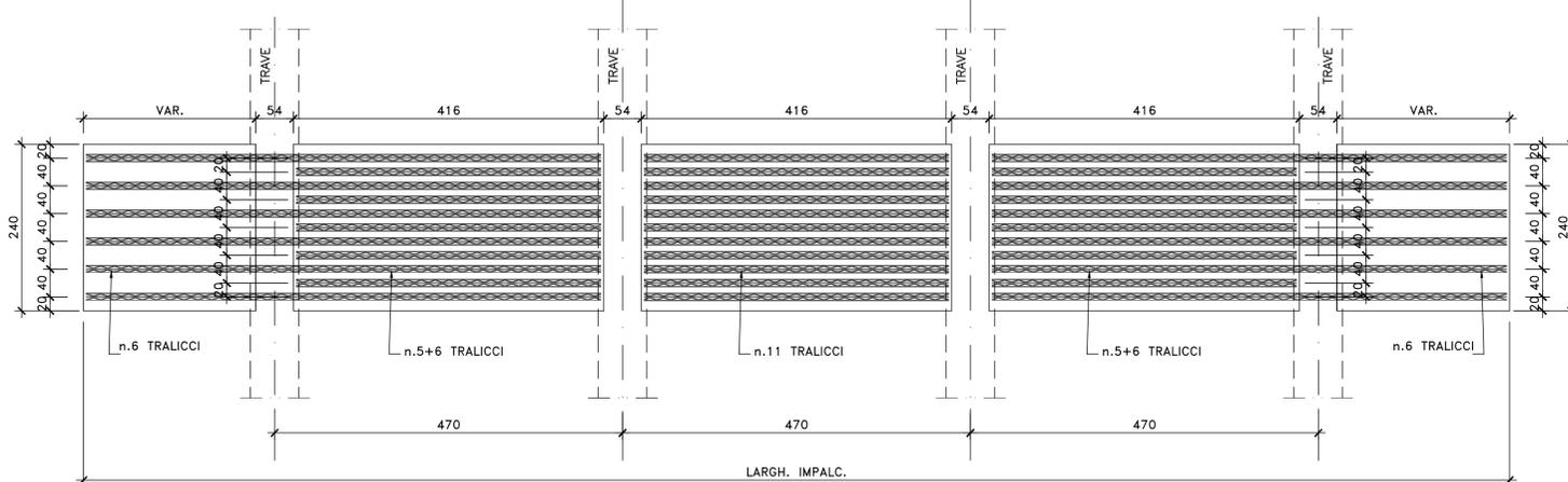
DETTAGLIO TIPOLOGICO APPOGGIO PREDALLE IMPALCATO (DX) A 3 TRAVI
