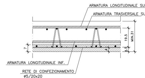
DETTAGLIO TIPOLOGICO APPOGGIO PREDALLE IMPALCATO (SX) A 4 TRAVI
