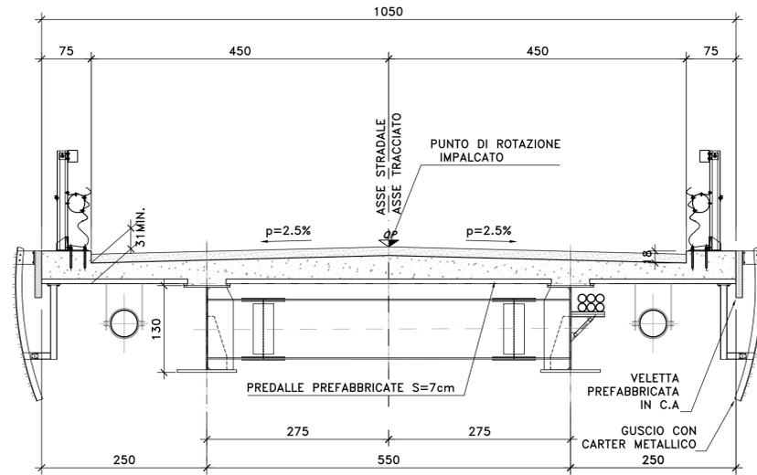
DETTAGLIO TIPOLOGICO APPOGGIO PREDALLE IMPALCATO B=10.50m
