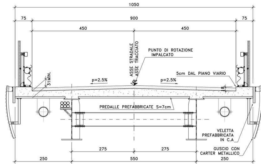
DETTAGLIO TIPOLOGICO APPOGGIO PREDALLE IMPALCATO B=10.50m
