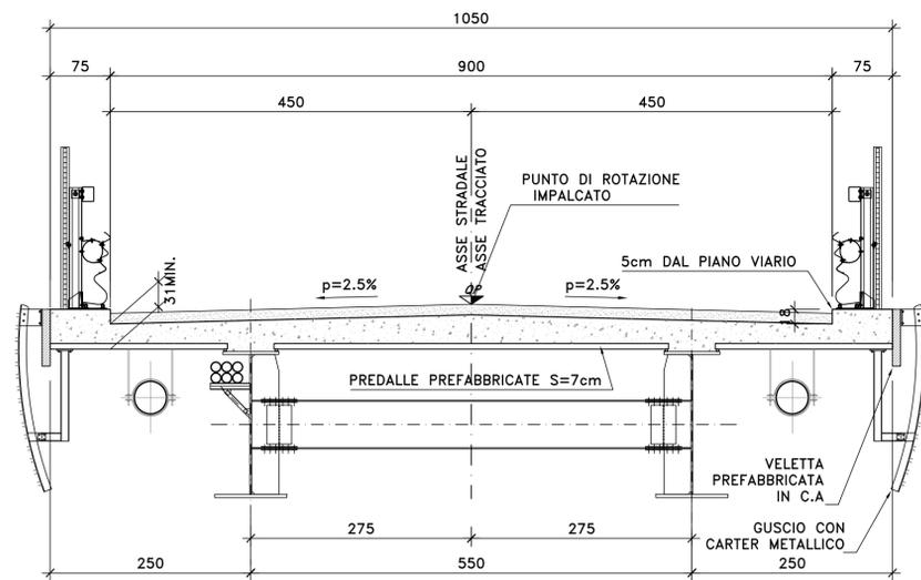
DETTAGLIO TIPOLOGICO APPOGGIO PREDALLE IMPALCATO B=10.50m
