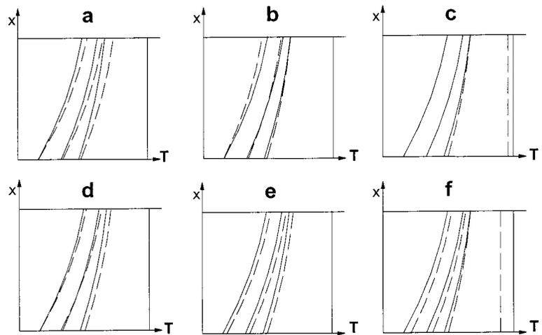
**Fig. 6 Temperature–heat-transfer area diagrams showing different situations in the simplified cooling circuit of Fig. 5. Temperature profiles have the same meaning of Fig. 5: from left, they refer to coolant, inner blade wall, outer blade wall, main gas stream. The continuous lines refer to the original situation, the dashed ones to modified conditions.**
