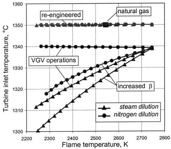
Fig. 7c: Total temperature at first rotor inlet (TIT)
