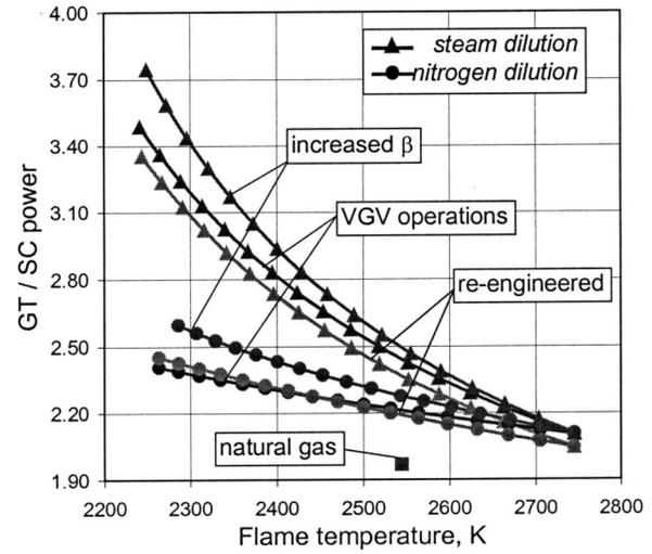
Fig. 7f: Gas turbine / steam cycle power output
