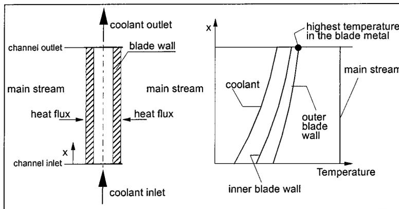
**Fig. 5 Simplified blade cooling model. Blade is assumed as a cross-flow heat exchanger where heat capacity of the outer stream is infinitely larger than the one of the inner stream. Main temperature profiles are reported in the right diagram.**
