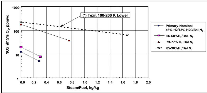
Figure 11: H<sub>2</sub> Syngas NO<sub>x</sub> Emissions as a Function of Steam/Fuel Mass Ratio
