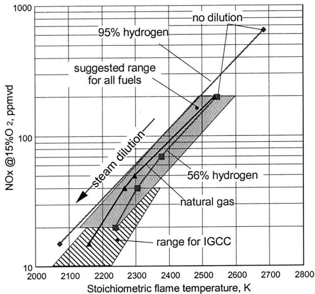
**Fig. 1** Relation between  $\text{NO}_x$  emission and stoichiometric flame temperature, progressively reduced by steam dilution, for gas turbine diffusive combustion at 12–16 bar with different fuels. Nitrogen is the balance gas for 56% and 95% hydrogen.
