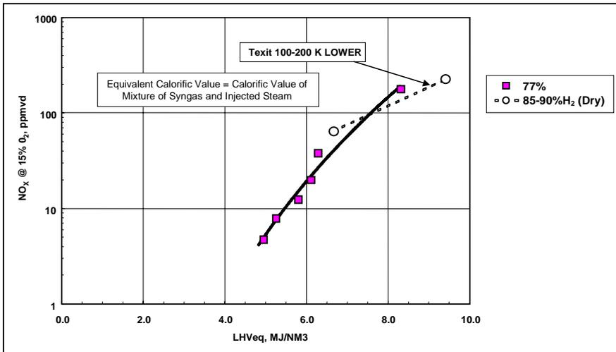
Figure 12: NO<sub>x</sub> vs Equivalent Calorific Value for Several Fuel Compositions
