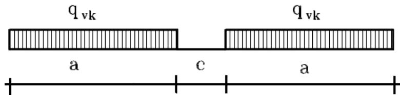
$$q_{\text{equivalente}} = 150 / 2.4 = 62.5 \text{ kN/m}^2$$
