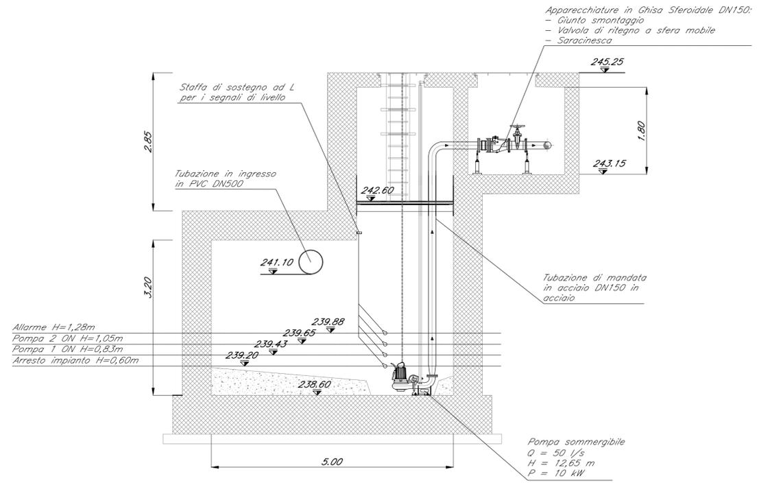
Apparecchiature in Ghisa Sferoidale DN150:
