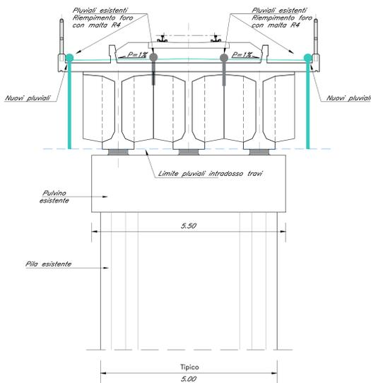
POZZETTO E GRIGLIE PARAFOLGIE PER PLUVIALI
