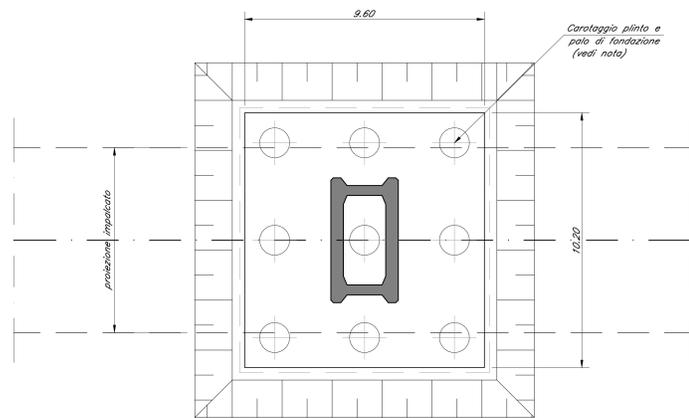
PIANTA SCAVI PILA A 9 PALI
