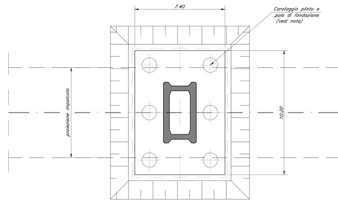
PIANTA SCAVI PILA A 6 PALI
