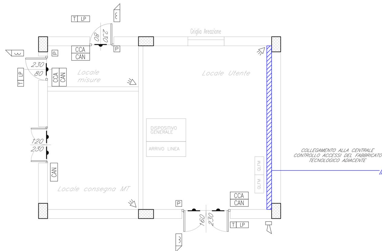
LAYOUT IMPIANTO ANTINTRUSIONE / CONTROLLO ACCESSI
