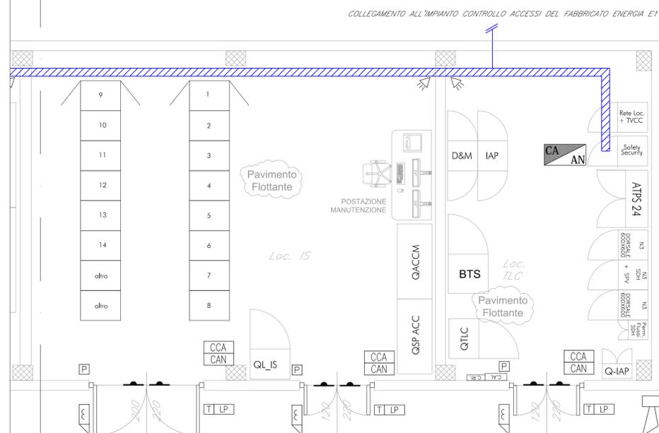
LAYOUT IMPIANTO ANTINTRUSIONE / CONTROLLO ACCESSI
