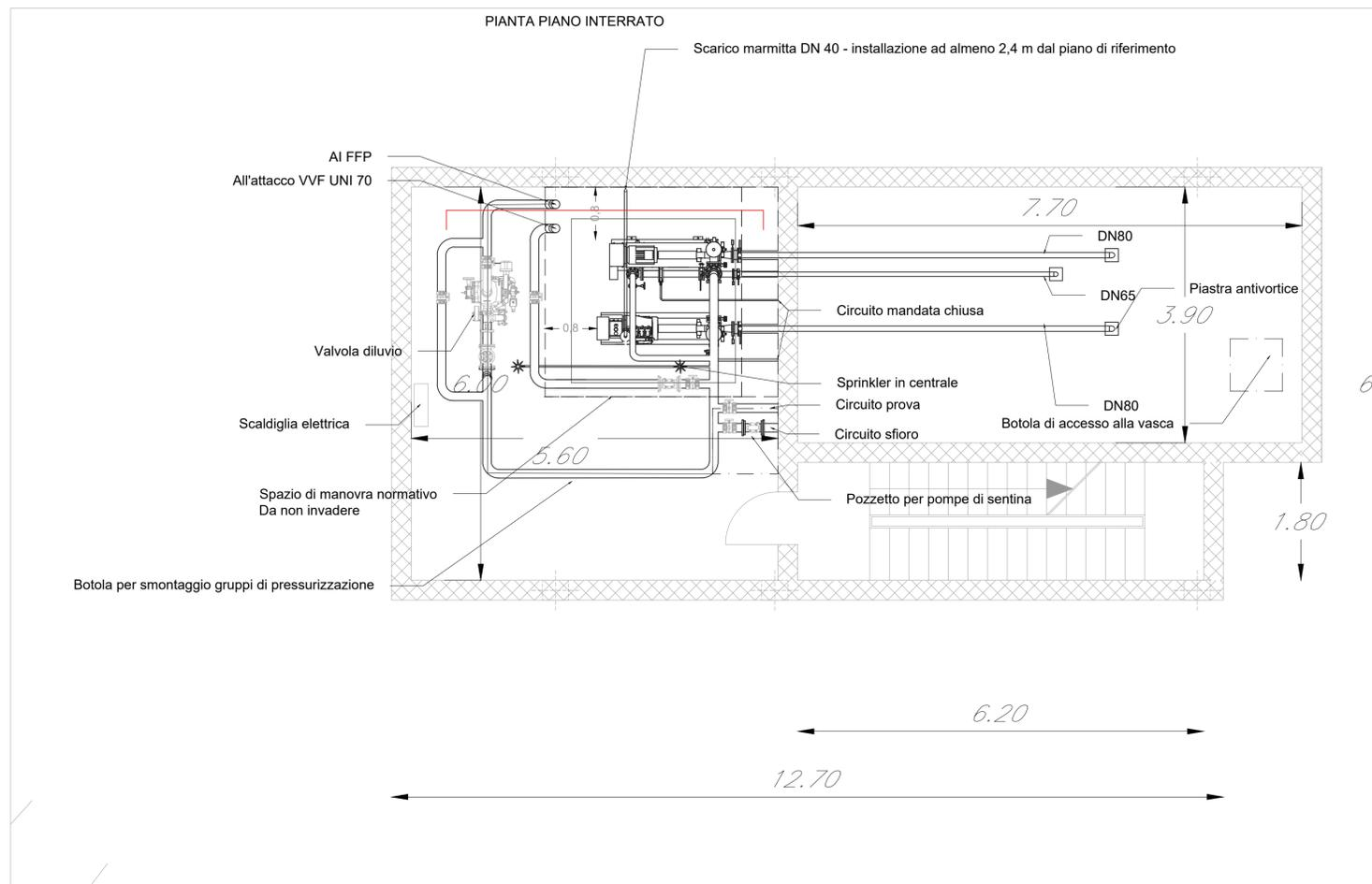
NOTA: IL LAYOUT TIPOLOGICO DELLA CENTRALE DI POMPAGGIO E' VALIDO PER I 3 PUNTIO ANTINCENDIO FFP01, FFP02, FFP03.
