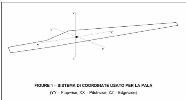
FIGURE 1 – SISTEMA DI COORDINATE USATO PER LA PALA
