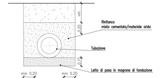
**SISTEMA DI DRENAGGIO IN TRINCEA PER TUBI FINO A D=200mm**
