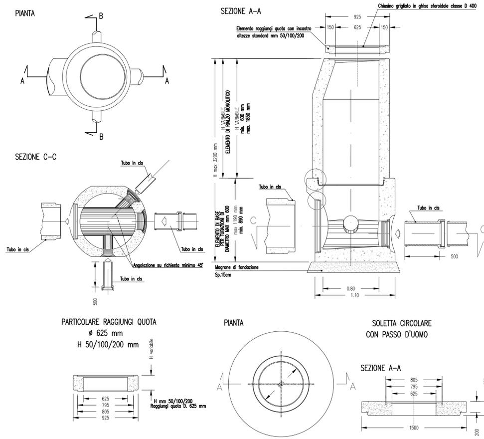
**SEZIONE TIPO DI POSA PER RACCORDO CADITOIE STRADALI (PVC DN200mm)**
