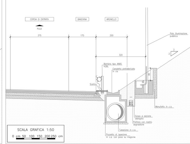
PARTICOLARE ELEMENTO MARGINALE CON BORDURA IN CORRISPONDENZA DEL PALO LUCE CON COLLETTORE Ø 800
