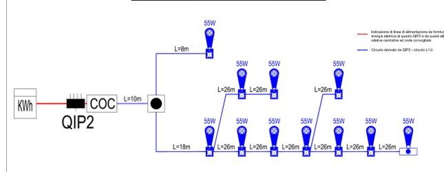
SCHEMA A BLOCCHI - ROTATORIA C
