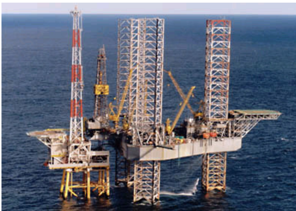
Fig. 3.1/1 – Jack-up drilling unit
