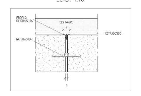
ELEMENTI WATER-STOP PER LA TENUTA IDRAULICA DEI GIUNTI SCALA 1:10
