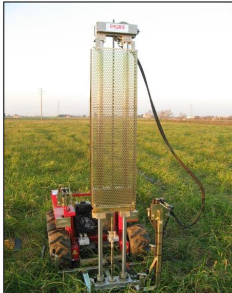
Fig.12: Penetrometro dinamico continuo (DPM – PAGANI Geotechnical Equipment)
