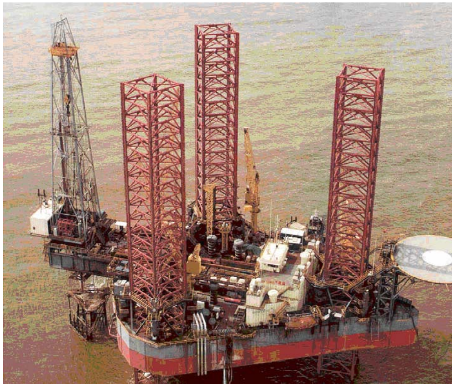
Figura 1.5- Jack-Up Drilling Unit
