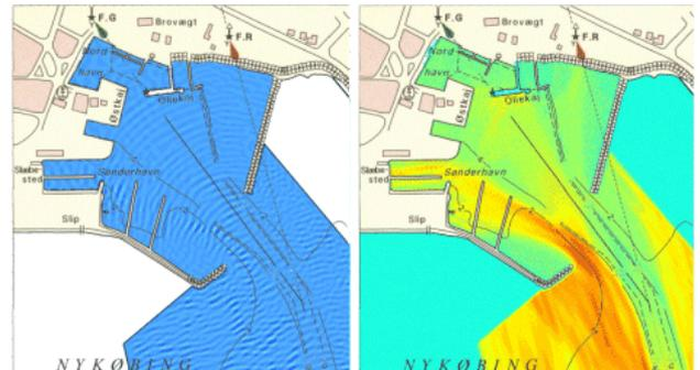
Output from MIKE 21 BW 2DH. The panel to the left shows a map of the instantaneous surface elevation. The right panel shows the map of the corresponding wave disturbance coefficients. Nykøbing Mors harbour, Denmark
