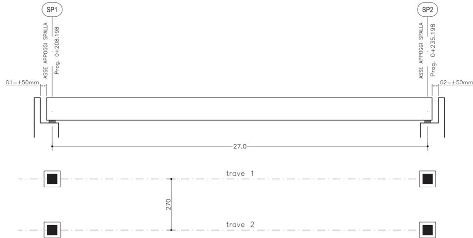
DISPOSITIVO DI APPOGGIO IN ELASTOMERO ARMATO
