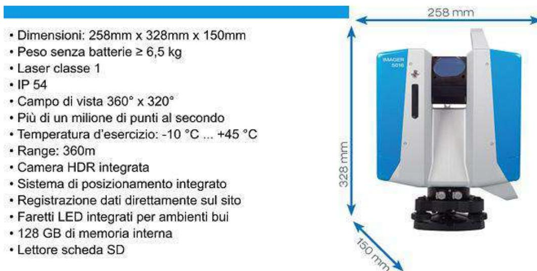
Figura 13 - Laser scanner Z+F-IMAGER-5016.
