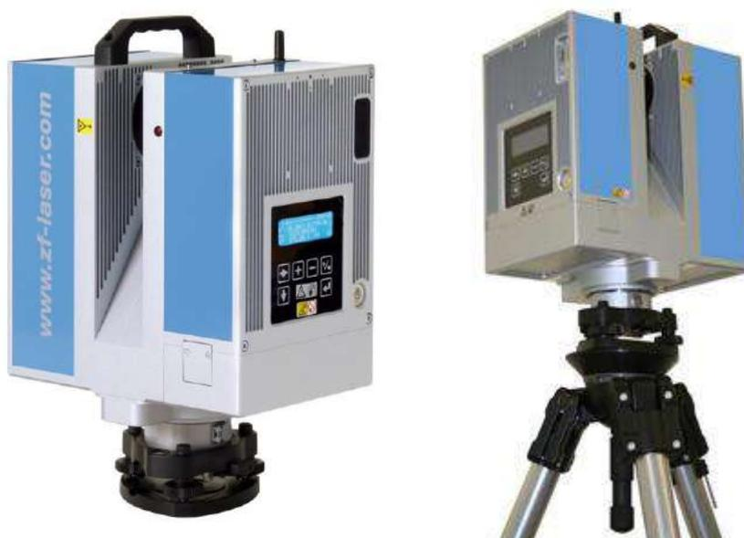
Figura 10 - Laser scanner Z+F-IMAGER-5006h
