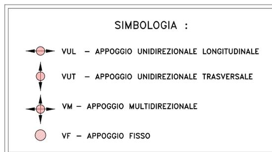
APPARECCHI DI APPOGGIO IN ACCIAIO-TEFLON A DISCO ELASTOMERICO CONFINATO
