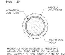
MICROPALI #300 INIETTATI A PRESSIONE ARMATI CON TUBO METALLICO VALVOLATI CON VALVOLE DI NON RITORNO OGNI 50 CM
