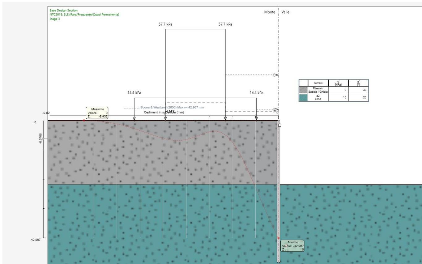
$$\delta = 9.92 - 4.34 = 5.58 \text{ mm} = 0.558 \text{ mm} < \delta_{\text{max, ammissibile}} = 1.35 \text{ cm}$$
