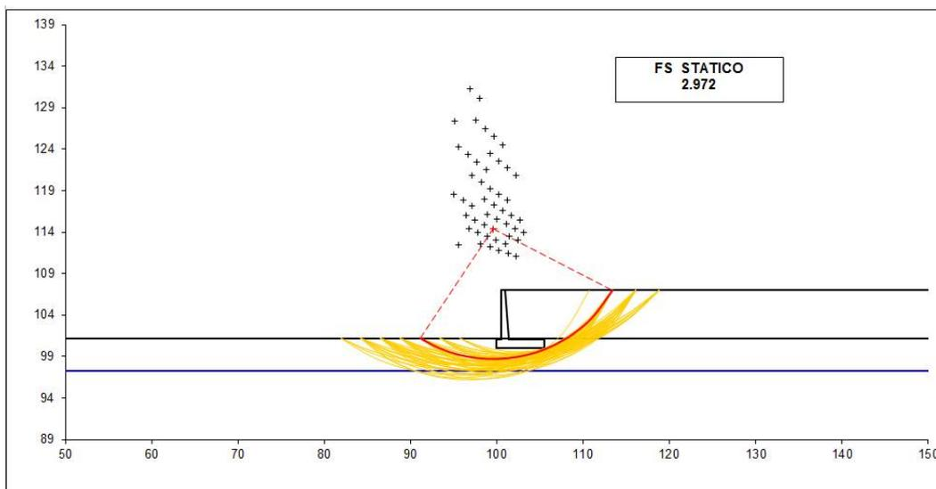
NV53A: MURO DI SOSTEGNO MU80B
