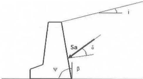
$$\text{per } i \leq \varphi' - \theta \quad k_a = \frac{\text{sen}^2(\psi + \varphi' - \theta)}{\cos \theta \text{sen}^2 \psi \text{sen}(\psi - \theta - \delta) \left[ 1 + \sqrt{\frac{\text{sen}(\varphi' + \delta) \text{sen}(\varphi' - i - \theta)}{\text{sen}(\psi - \theta - \delta) \text{sen}(\psi + i)}} \right]^2}$$
