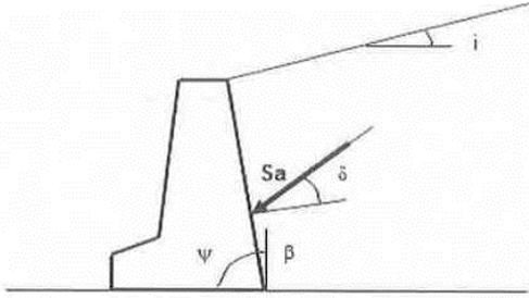
$$\text{per } i \leq \varphi' - \theta \quad k_a = \frac{\text{sen}^2(\psi + \varphi' - \theta)}{\cos \theta \text{sen}^2 \psi \text{sen}(\psi - \theta - \delta) \left[ 1 + \frac{\text{sen}(\varphi' + \delta) \text{sen}(\varphi' - i - \theta)}{\text{sen}(\psi - \theta - \delta) \text{sen}(\psi + i)} \right]^2}$$
