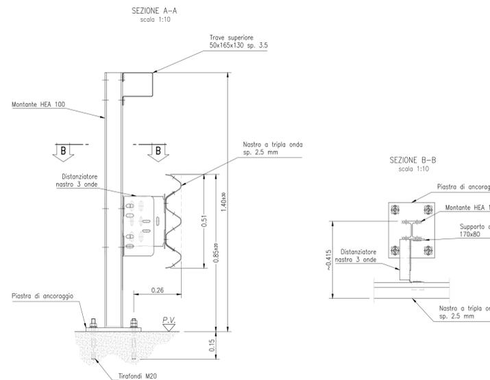
BARRIERA TIPO "H2W4" - RILEVATO
