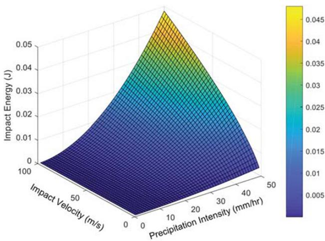
**FIGURE 2** Raindrop impact energies as a function of impact velocity and rainfall rate [Colour figure can be viewed at [wileyonlinelibrary.com](http://wileyonlinelibrary.com)]
