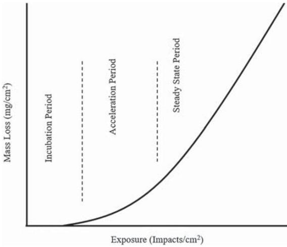
**FIGURE 3** Erosion timeline for liquid droplet impingement
