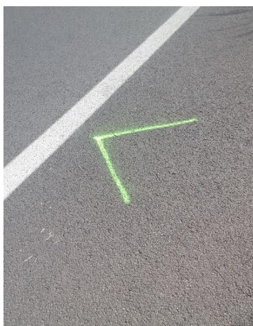
Figura 6 - Gruound Control Point (GCP).
