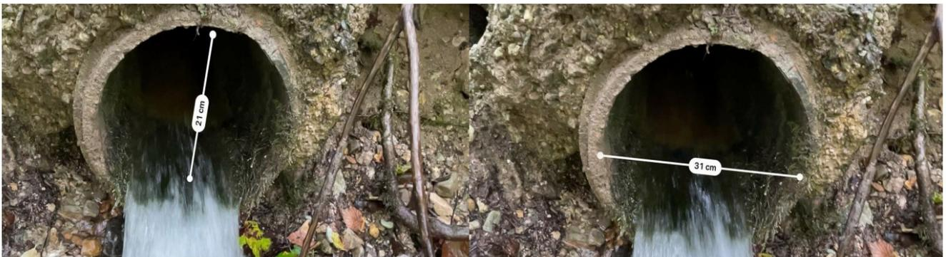
**D1:** the pipe draining water from Ponente portal to Vedra river. Water measurements have been made with barrel and chronometer.
