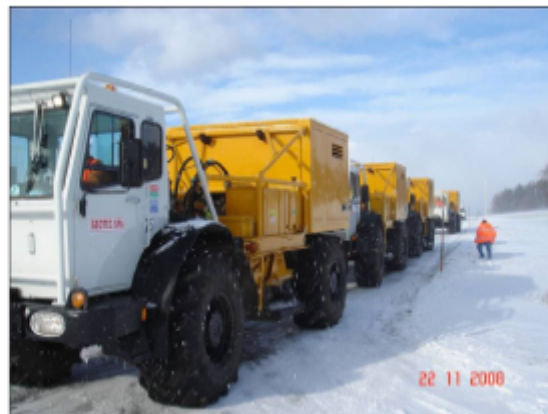
VIBRATOR UNIT VVCA/E WITH SILENT PACK
