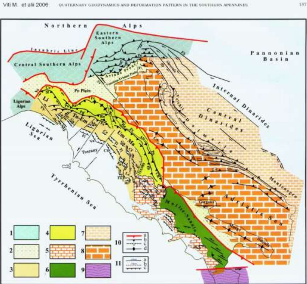
Fig. 4 - Main structural and tectonic features in the Central-Northern Apennines and the northern peri-Adriatic zones. 1) Ligurian and Southern Alps; 2) Foredeep basins; 3, 4) Axial and outer belts of the Northern Apennines; 5) Latium-Abruzzi and Southern Apennines carbonate platforms; 6) Outer belt of the Southern Apennines; 7) Dinarides carbonate platforms; 8) Adriatic foreland; 9) Calabrian Arc; 10) Compressional features: a = outer front of the Alps and Apennines; b,c = active and inactive thrusts; d = fold axes; 11) Transcurrent and extensional features: a, b = active and presumably active strike-slip faults; c = normal faults. Main compressional features: CA = central Adriatic folds; Co = San Colombano-Cremona; CR = Coastal Ridge; Fa = Faenza; Fe = Ferrara; IR = Internal Ridge; OAMS = Olevano-Antrosdoco-Monti Sibillini lineament; Pa = Parma; Pd = Pedepennine; Pe = Periadriatic; Po = Porto S. Giorgio, Re = Reggio Emilia; Ro = Romagna; Ri-Pe-An = Rimini-Pesaro-Ancona; St = Stradella-Florenzuola d'Arda; Vo = Voghera-Pavia. Main strike-slip features: EN = Enza; FS = Fella-Sava; ID = Idria; RJ = Rijeka; SV = Schio-Vicenza; VV = Villaverzia-Varzi. Main extensional/transensional basins: Aq = Aquila; Ca = Casentino; Ch = Chiana; Cf = Colfiorito; Fi = Firenze-Pistoia; Fo = Foligno-Spoleto; Fu = Fucino; Ga = Garfagnana; Gu = Gubbio; Le = Leonessa; Lu = Lunigiana; Mg = Magra; Mu = Mugello; No = Norcia; Ri = Rieti; Sg = Upper Sangro; Su = Sulmona; Ti = Tevere; Tn = Terni; Va = Valdarno; Li = Ligurian Apennines; Mi = Maiella; Tl = Tagliamento river; Tu-Em = Tuscany-Emilia Apennines; Um-Ma = Umbria-Marche Apennines. Details on tectonic features in the Southern Apennines are given in Figs 1 and 3. See text for explanations.
