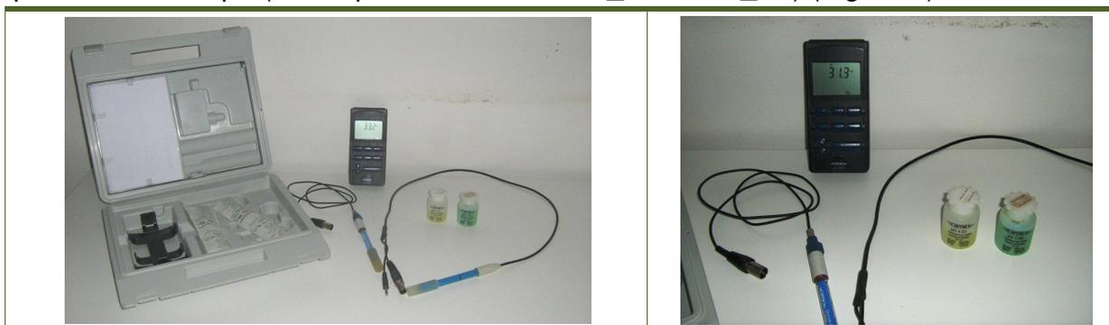
Figura 5. pHmetro portatile WTW pH 330i
