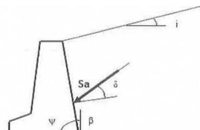
$$\text{per } i \leq \varphi' - \theta \quad k_a = \frac{\text{sen}^2(\psi + \varphi' - \theta)}{\cos \theta \text{sen}^2 \psi \text{sen}(\psi - \theta - \delta) \left[ 1 + \frac{\text{sen}(\varphi' + \delta) \text{sen}(\varphi' - i - \theta)}{\sqrt{\text{sen}(\psi - \theta - \delta) \text{sen}(\psi + i)}} \right]^2}$$
