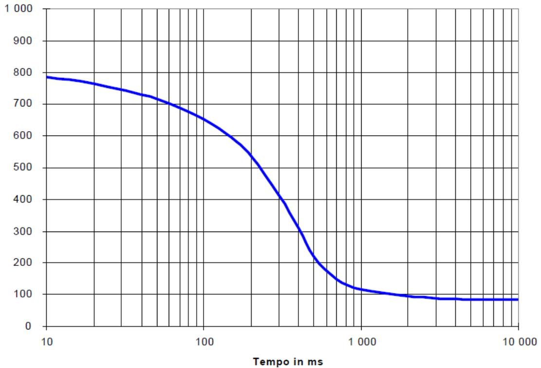
Figura 4 – Curva Tempo-Tensione (Norma CEI EN 50522 § 5.4.3)
