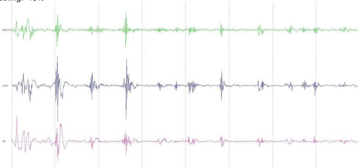
Max. H/V at 63.97 ± 14.19 Hz. Max (N-S)/V: 30.94 ± 19.95 Hz. Max (E-W)/V: 59.63 ± 13.31 Hz. (In the range 0.0 - 64.0 Hz)
