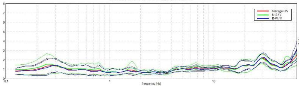
**HORIZONTAL TO VERTICAL SPECTRAL RATIO**
