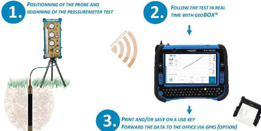
Conformed to procedure B of ISO 22476-4 standard, recordings are automatically carried out after 1, 15, 30 and 60 seconds with optimized accuracy: 0,1 cm<sup>3</sup> on the volume and 10 kPa on the pressures.
