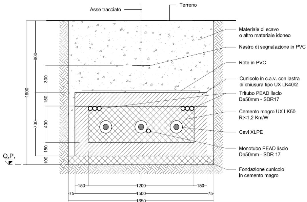
Figura 7.7/12 – Posa in cunicolo in cemento armato – cavo 245 kV e 420 kV in piano
