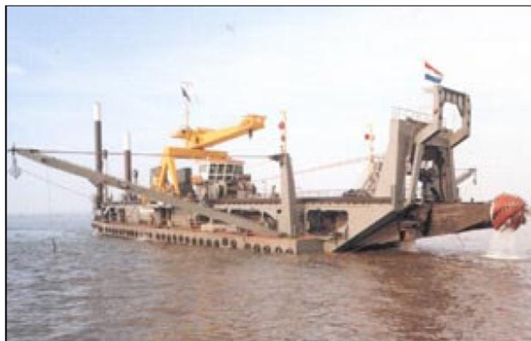
*Figura 4.6: cutter suction dredger – CSD*
